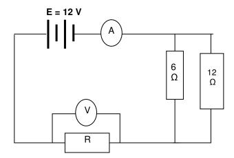
If the reading on the voltmeter is 4  $\mathbf{V}$ , what will the reading on the ammeter be?
