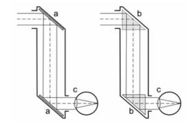
Principle of the periscope: The periscope on the left uses mirrors at location "a" whereas the right uses prisms at "b". The observer is "c".
