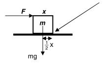
When the torque (moment of the force) produced by the applied force F is just enough to topple the block, the toppling torque due to F is equal to the restoring torque due to mg about the edge shown:
