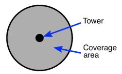
When the coverage area of two towers overlaps the towers are said to be directly connected. Towers can also be indirectly connected if there is a chain of directly connected towers between the two towers.
